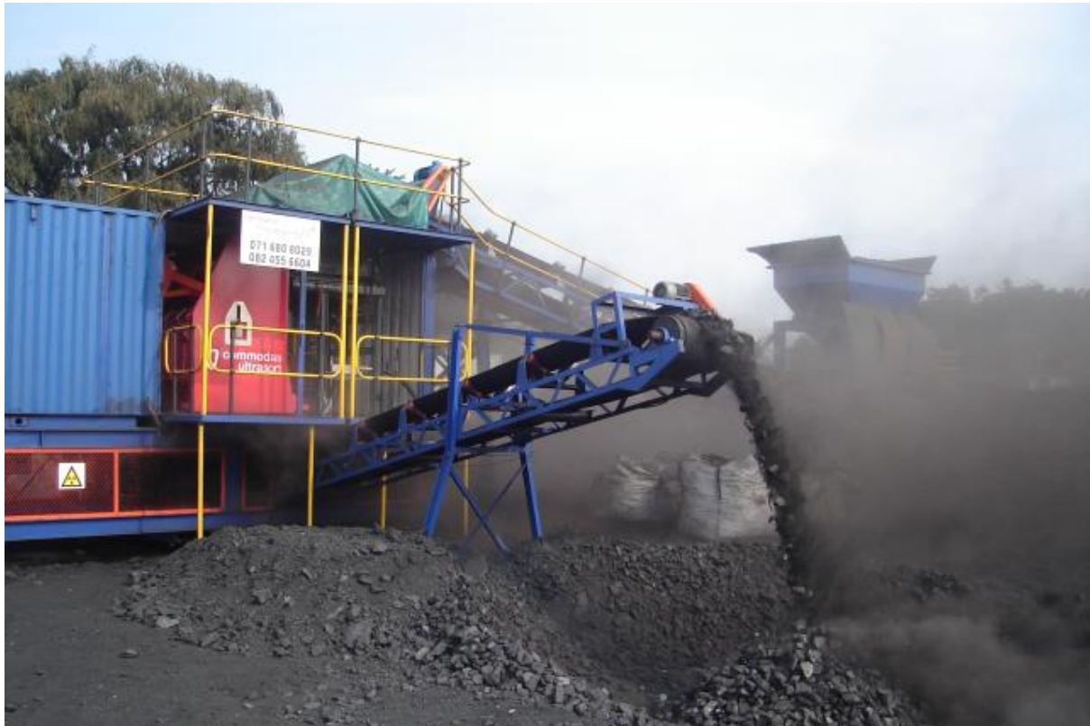
Figure 6: X-ray sorter in operation
