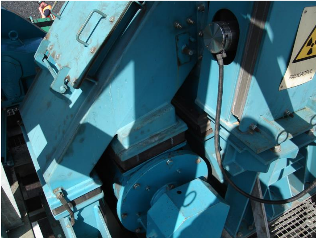
Figure 8: Density gauge and star gate for controlled removal of discard
